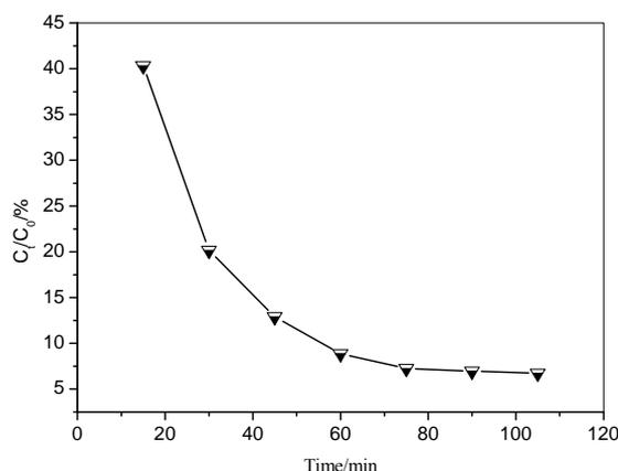
Figure 5. Desorption curve for MB adsorption on IOPCPF.
