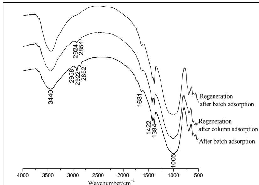
Figure 9. FTIR curves of regeneration of IOPCPF after absorbed MB.
