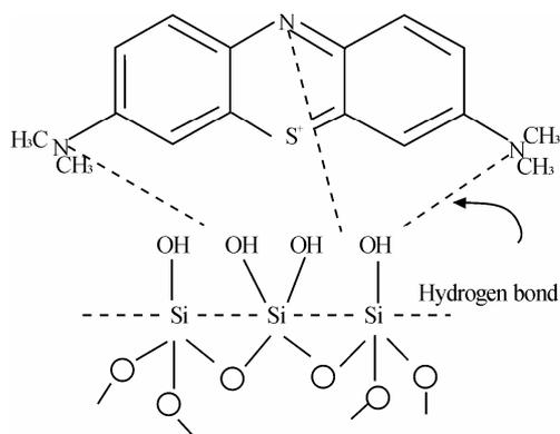
Figure 8. Hydrogen bond formation between adsorbent and MB.
