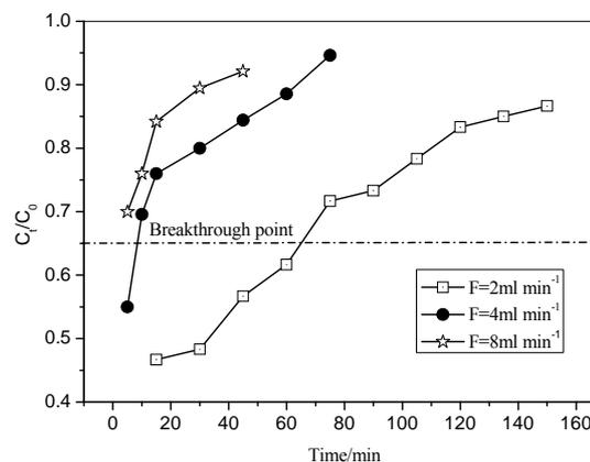
Figure 4. Breakthrough curves for MB adsorption on IOPCPF at different flow rate.
