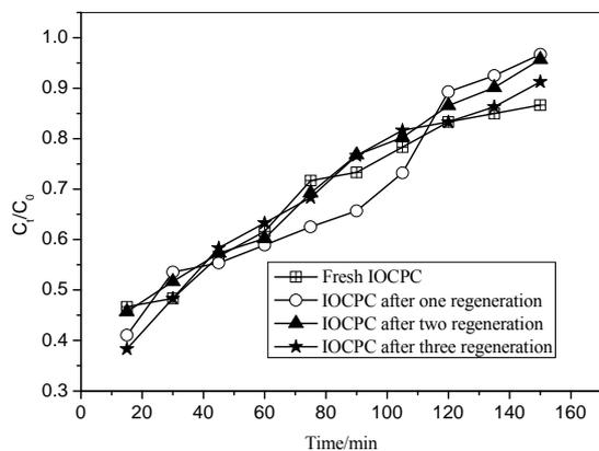
Figure 6. Recycling of regenerative adsorption column.
