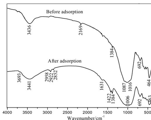
Figure 7. Infrared spectra of IOCPFC before and after adsorbed MB (MB initial concentration: 100mg/L, Temperature: 30°C).
