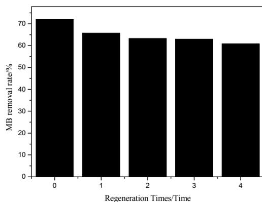
Figure 3. Effect of regeneration cycles on MB removal rate of IOPCPF.
