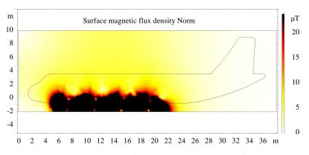
Figure 12. Magnetic induction around the mid-size passenger aircraft accelerating by maglev technology.
