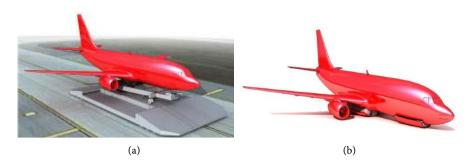
**Figure 13.** Landing of undercarriage-less aircraft on the ground moving cars (on own wheels) or on the lightweight skids (opening for forced landing).
