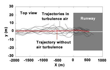
**Figure 7.** Simulated GABRIEL automatic landing aircraft trajectories for scenarios without turbulence (red) and with turbulence (black, 10 simulations) in 25 knots lateral crosswind.
