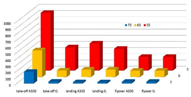
**Figure 3.** Areas (in km<sup>2</sup>) effected by single aircraft flight phases (vertical axis), at 55, 65 and 75 SEL Sound Exposure Level) noise (in dB) defined for reference A320 and G. - Gabriel aircraft (best optimized trajectory).
