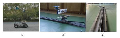
**Figure 8.** The practical concept validation tests: (a) UAV landing on electric car; (b) developed test track; (c) landing of the validation model on test track.
