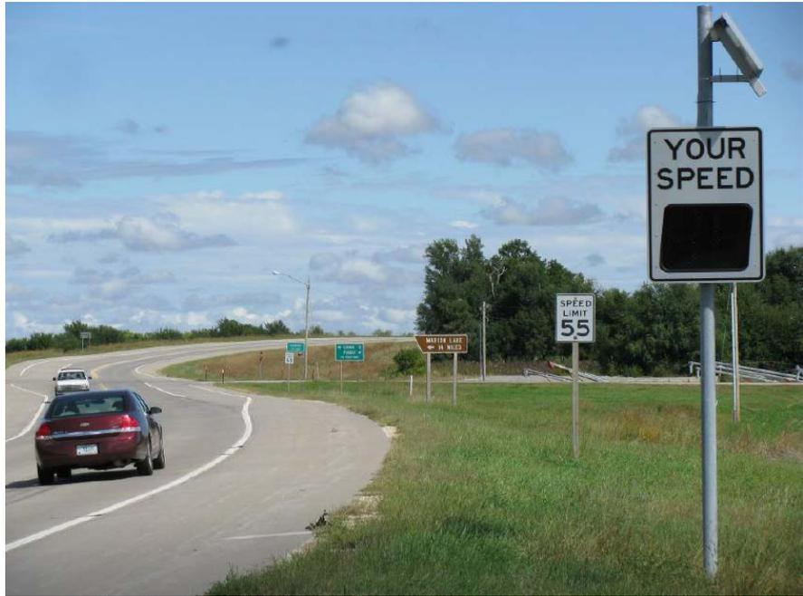
**Figure 1.** Solar speed display at west city limit, peabody (photo by Joe Palic).
