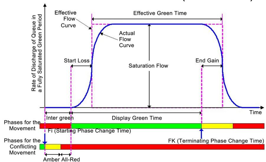
**Figure 4.** Basic model of saturation flow rate, (Source HCM 2000).
