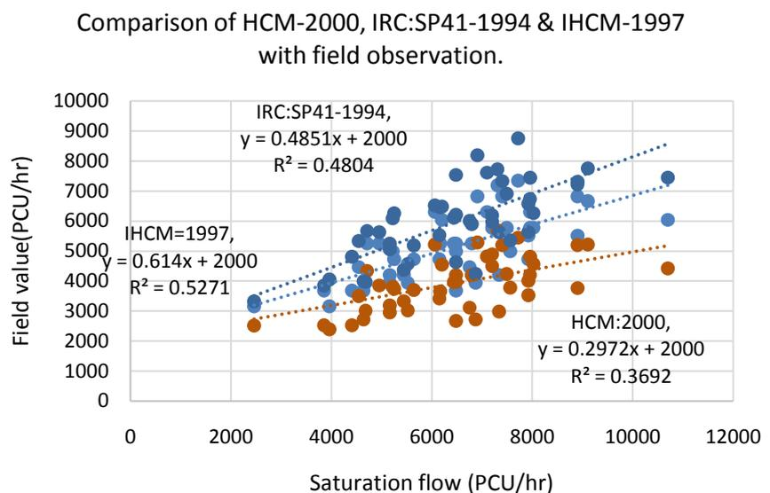
Figure 5. Comparison of field value with HCM-2000, IHCM-1997, IRC: SP41-1994.
