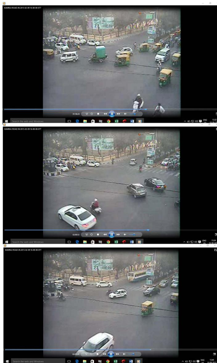
**Figure 3.** Traffic data collection for a typical junction by videography.
