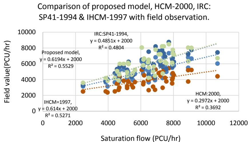
**Figure 6.** Comparison of saturation flow rate by IRC method & proposed model.
