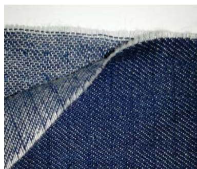
Figure 2. Visual appearance of double cloth.
