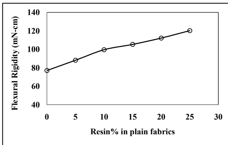
**Figure 4.** Flexural rigidity of polyester resin treated jute plain fabrics.
