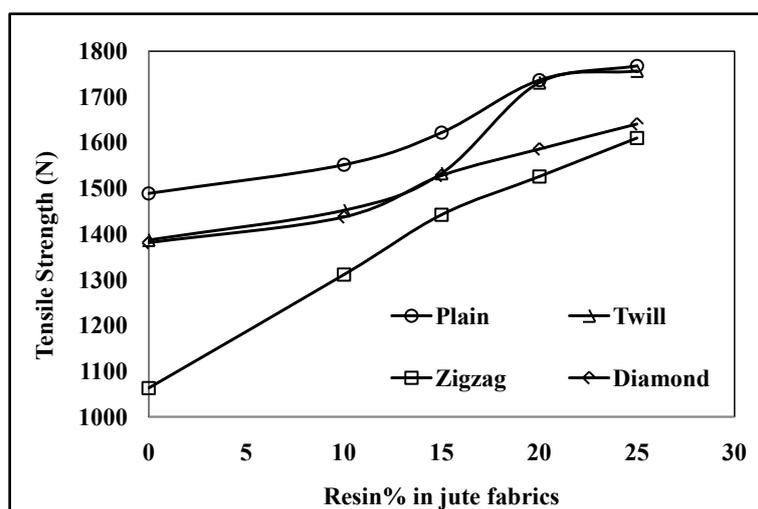
**Figure 7.** Effect of polyester resin treatment on the tensile strength of plain, twill, zigzag and diamond structure of jute fabrics.
