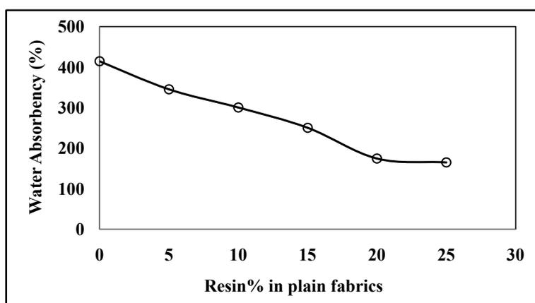
**Figure 2.** Water absorbency (%) of polyester resin treated jute plain fabrics.
