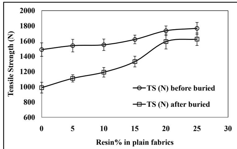
**Figure 6.** Tensile strength of polyester resin treated jute plain fabrics before and after buried into soil.
