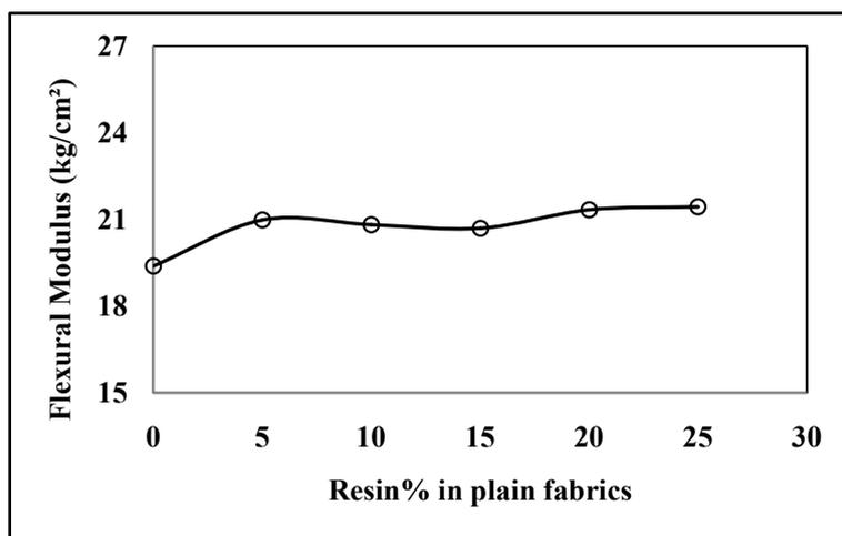
**Figure 5.** Flexural modulus of polyester resin treated jute plain fabrics.
