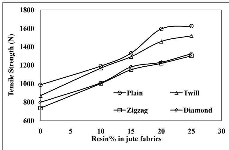
**Figure 8.** Effect of soil degradation on the tensile strength of polyester resin treated plain, twill, zigzag and diamond structure of jute fabrics.
