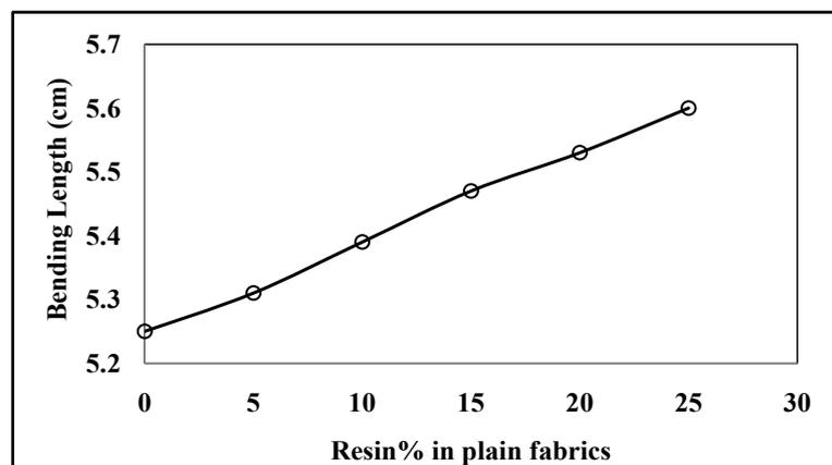
**Figure 3.** Bending length of polyester resin treated jute plain fabrics.
