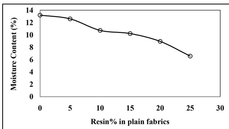
**Figure 1.** Moisture content (%) of polyester resin treated jute plain fabrics.
