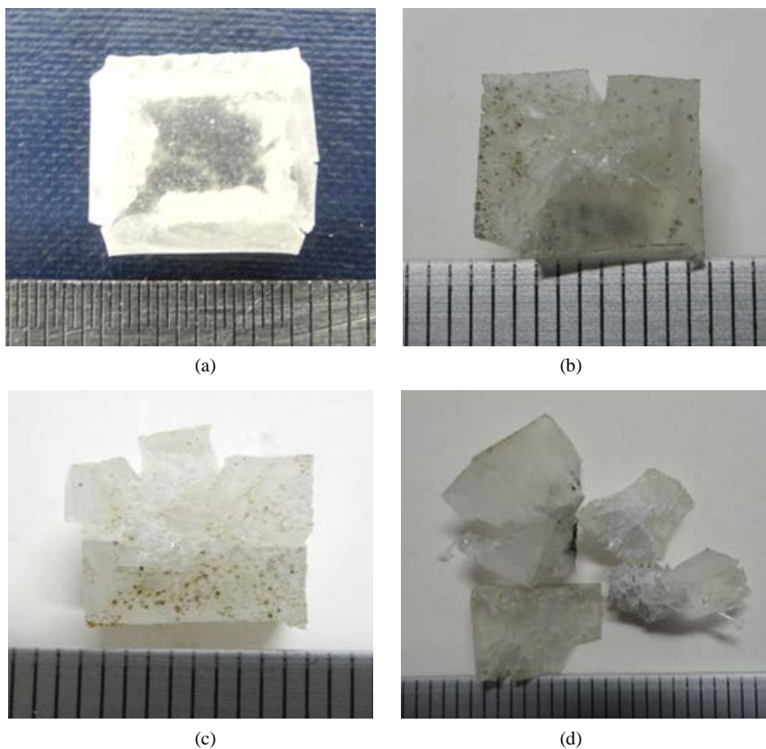
Figure 11. Compression fractures of epoxy/SiO 2 (0 wt%) composites at various strain rates. (a) 0.001/s; (b) 800/s; (c) 1400/s; (d) 2000/s.
