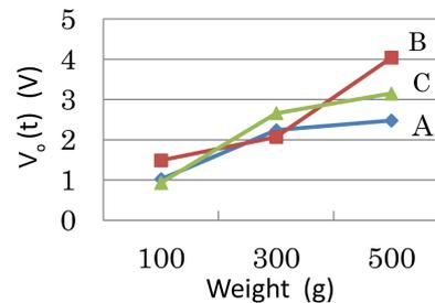
**Figure 6.** The dependence of the weight loaded on the rubber sheet sensor on the output voltage  $V_o$ . The signs A, B and C refer to Sample A, B and C, respectively.
