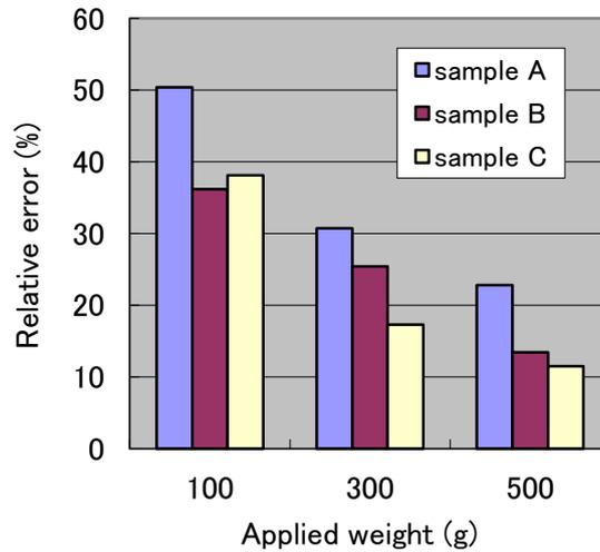
**Figure 5.** Relative errors reduce with the applied weight. It shows at the same time that Sample C comparatively gives small error in general.
