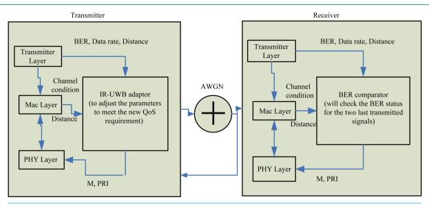
Figure 4. Proposed architecture for adaptive UWB-RFID communication model
