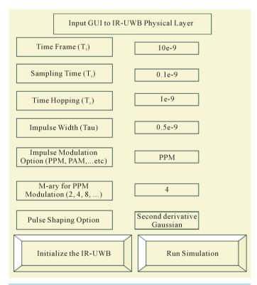
Figure 7. Graphical user interface showing different IR-UWB PHY parameter settings.
