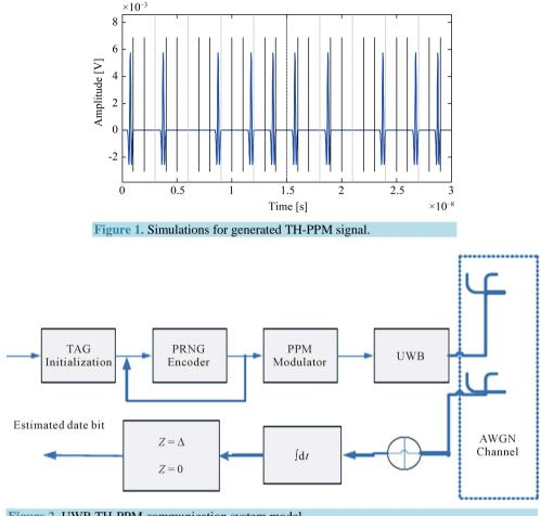
Figure 2. UWB TH-PPM communication system model.
