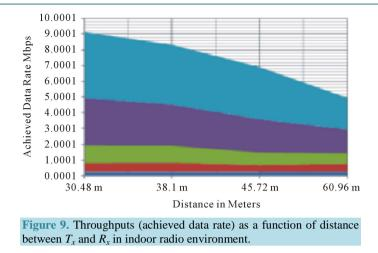
power level of -12.2 dBm (approximately 50% packet drops). At an extreme distance of 61 meters, the throughput decreases significantly, as higher data rate is more exposed to interferences and multipath effects. Also, the signal power attenuated due to the extended ranges.
