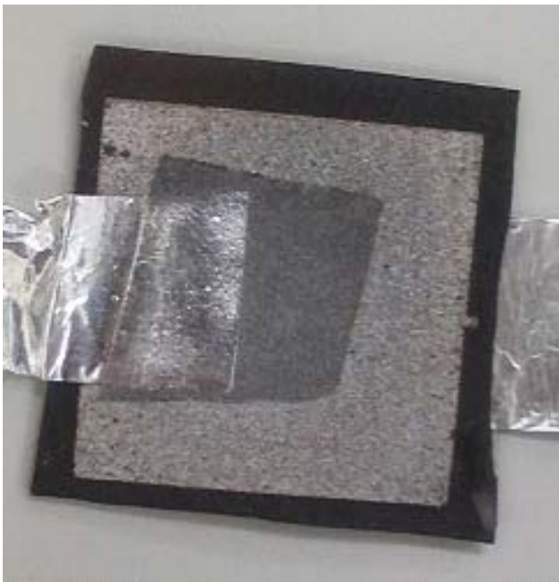
Figure 1. The outlook of the rubber sheet sensor with aluminum electrode deposited on the surface. On the deposited aluminum, Al foil was attached as a conductor to a detecting circuit.
