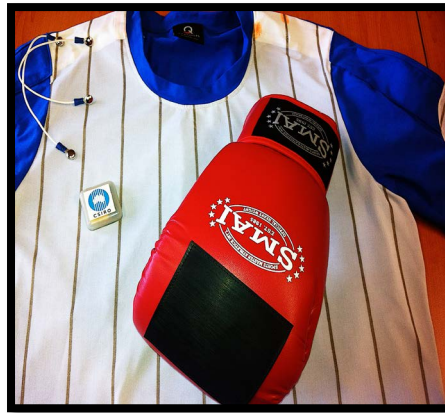
Figure 1. Components of the automated scoring system used in Box'Tag. The image shows an instrumented vest and a conductive patch on a glove. Wires connecting vest to transceiver also can be seen. When connected, the transceiver sits in a pocket on the upper back. Photograph provided by Kris Arnold Photography, Canberra, Australia.
