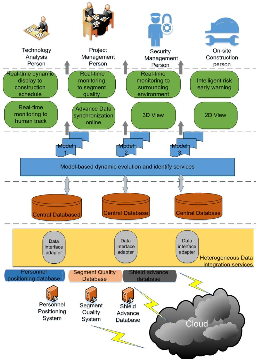
Figure 4. Cloud-based Open-BIM tunnel construction information system.
