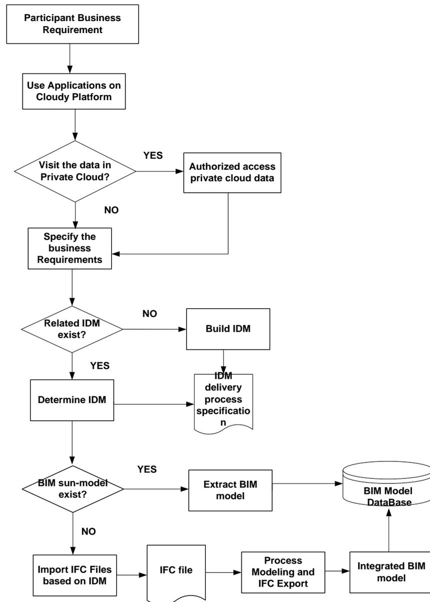
Figure 3. Cloud and open-based building information interoperability process.
