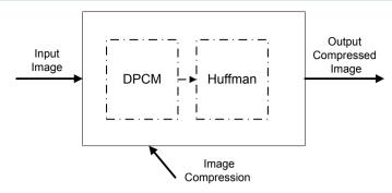
**Figure 3.** Schematic diagram of the image compression algorithm using DPCM-Huffman encoding.
