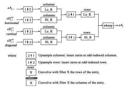
Figure 6. One level inverse 2D-DWT [20].
