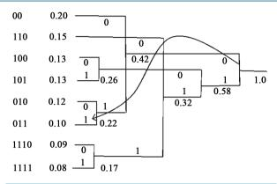
Figure 2. Huffman coding procedure [4].
