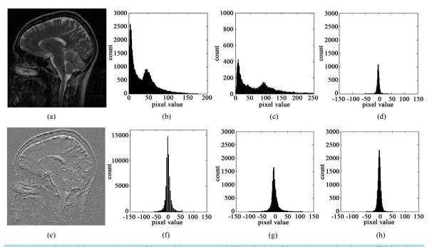
Figure 9. (a) Original image; (b) original image histogram; (c) DWT of original image (approximation coeffeicint) histogram; (d) DWT of original image (details coeffeicint) histogram; (e) DPCM output; (f) DPCM output histogram; (g) DWT of DPCM output (approximation coeffeicint) histogram; (h) DWT of DPCM output (details coeffeicint) histogram.
