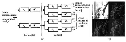
Figure 5. Filtering implementation of 2D-DWT [21].
