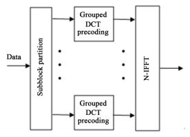
Figure 2. Block of the grouped DCT precoding scheme.
