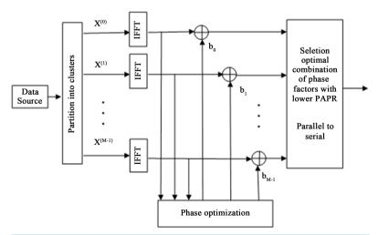
Figure 1. Block diagram of conventional PTS-OFDM scheme.
