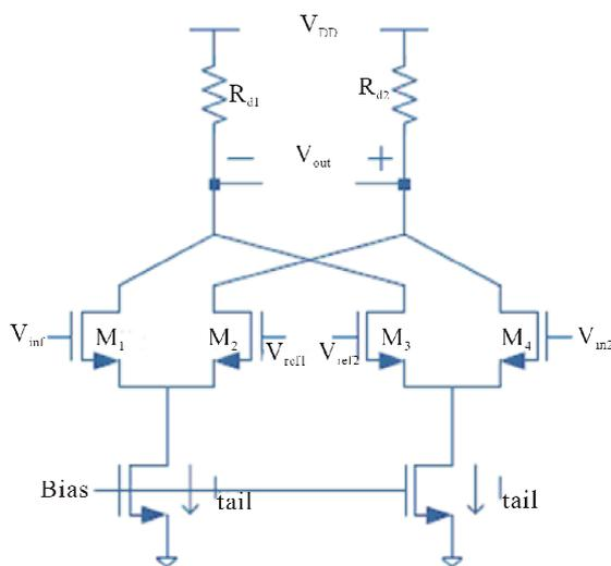
**Figure 1. Schematic of the preamplifier.**
