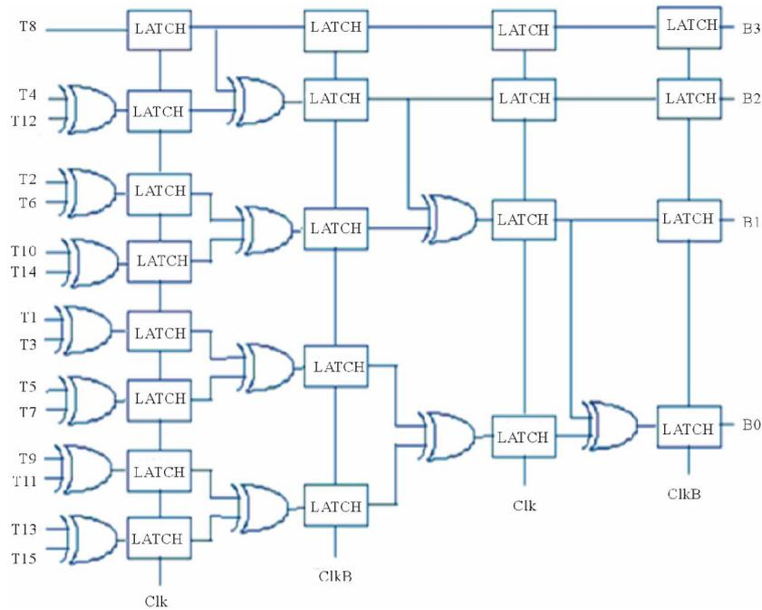
Figure 2. Implementation of encoder with four stage pipeline and only one type of gate.
