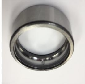
Figure 3. Outer race fault.
