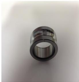
Figure 4. Inner race fault.
