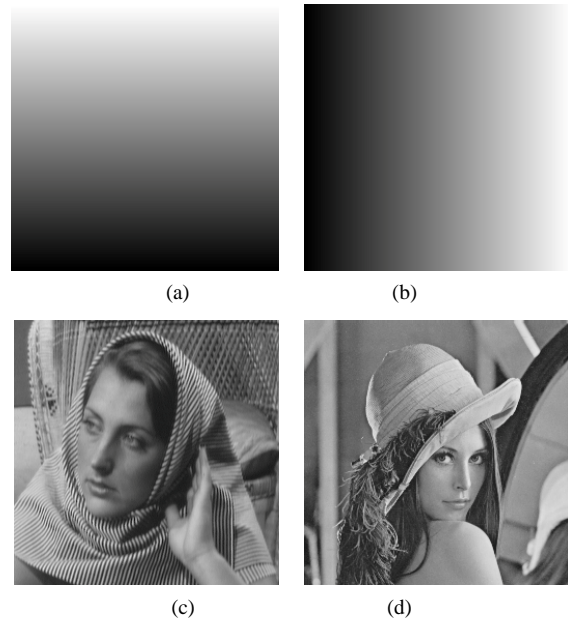
Figure 4. Examples of 8-bit source images of 256 by 256 pixels used in the experiments: (a) Vertical ramp with 1-level per pixel gradation; (b) Horizontal ramp with 1-level per pixel gradation; (c) Barbara and (d) Lena .
