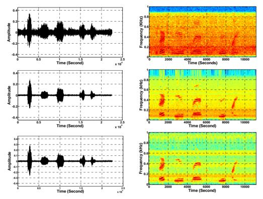
Figure 7. Temporal waveforms and speech spectrogram with sp1 utterance, "*The birch canoe slid on the smooth planks*", by a male speaker from the NOIZEUS speech corpus: (from top to bottom) noisy speech (degraded by car noise at 5 dB SNR); speech enhanced by MBSS (PESQ = 1.776), and speech enhanced by IP-MBSS (1.915).
