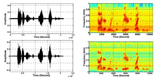
Figure 10. Temporal waveforms and speech spectrograms of sp10 utterance, "*The sky that morning was clear and bright blue*", by a male speaker from the NOIZEUS speech corpus: (from top to bottom) clean speech; noisy speech (speech degraded by car noise at 10 dB SNR); speech enhanced by MBSS (2.259); and speech enhanced by IP-MBSS (2.459).
