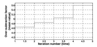
Figure 4. Variations of over-subtraction factor (mean value) with iteration times (number).
