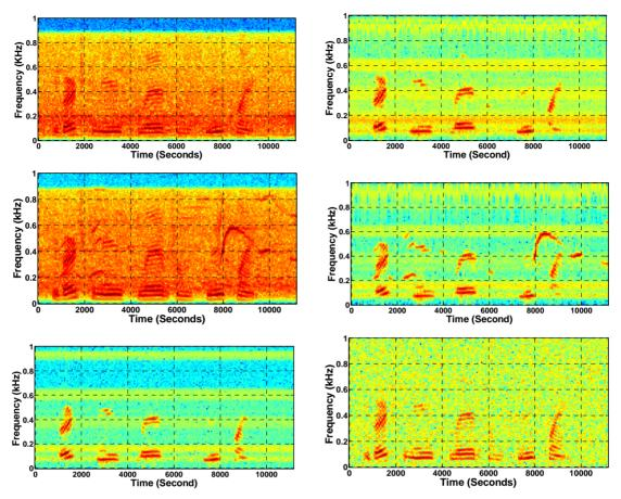
Figure 5. Speech spectrograms of sp1 utterance, "*The birch canoe slid on the smooth planks*", by a male speaker from the NOIZEUS speech corpus: (from top to bottom) clean speech; (left side, from top to bottom) speech degraded by car noise, train noise, babble noise, restaurant noise, airport, street, exhibition, and white noise, respectively (5 dB SNR); (right side, from top to bottom) corresponding enhanced speech.
