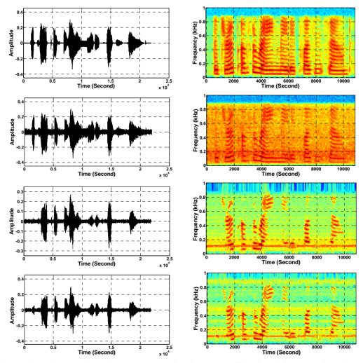
Figure 11. Temporal waveforms and speech spectrograms of sp12 utterance, *"The drip of the rain made a pleasant sound"*, by a female speaker from the NOIZEUS speech corpus: (from top to bottom) clean speech; noisy speech (degraded by car noise at 10 dB SNR); speech enhanced by MBSS algorithm (2.005); and speech enhanced by IP-MBSS (2.255).
