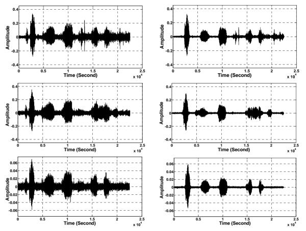
Figure 6. Temporal waveforms of sp1 utterance, "*The birch canoe slid on the smooth planks*", by a male speaker from the NOIZEUS speech corpus: (from top to bottom) clean speech; (left side, from top to bottom) speech degraded by car noise, train noise, babble noise, restaurant noise, airport noise, street noise, exhibition noise, and white noise, respectively (5 dB SNR); (right side, from top to bottom) corresponding enhanced speech.
