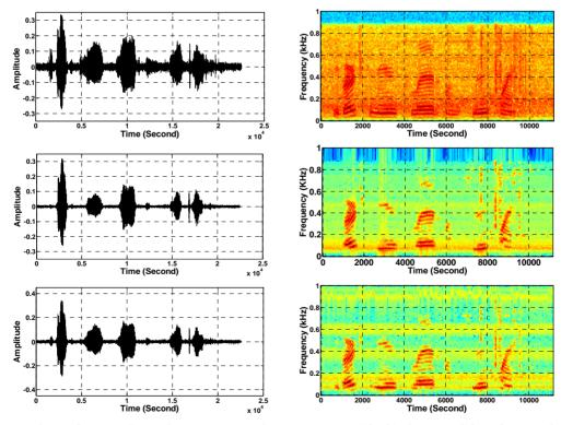
Figure 8. Temporal waveforms and speech spectrogram of sp1 utterance, "*The birch canoe slid on the smooth planks*", by a male speaker from the NOIZEUS speech corpus: (from top to bottom) noisy speech (degraded by car noise at 10 dB SNR); speech enhanced by MBSS (PESQ = 2.030), and speech enhanced by IP-MBSS (PESQ = 2.147).
