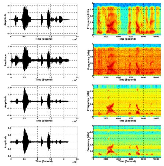
Figure 9. Temporal waveforms and speech spectrograms of sp 6 utterance, "*Men strive but seldom get rich*", by a male speaker from the NOIZEUS speech corpus: (from top to bottom) clean speech; noisy speech (speech degraded by car noise at 10 dB SNR); speech enhanced by MBSS algorithm (PESQ = 2.157); and speech enhanced by IP-MBSS (PESQ = 2.267).
