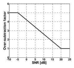
Figure 1. The relation between over-subtraction factor and SNR.
