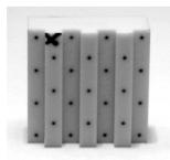
Figure 7. Two-level calibration target (dimensions: 20 mm  $\times$  20 mm  $\times$  5 mm; level height: 2 mm) with 25 reference points of known coordinates ( $\emptyset = 0.5$  mm).
