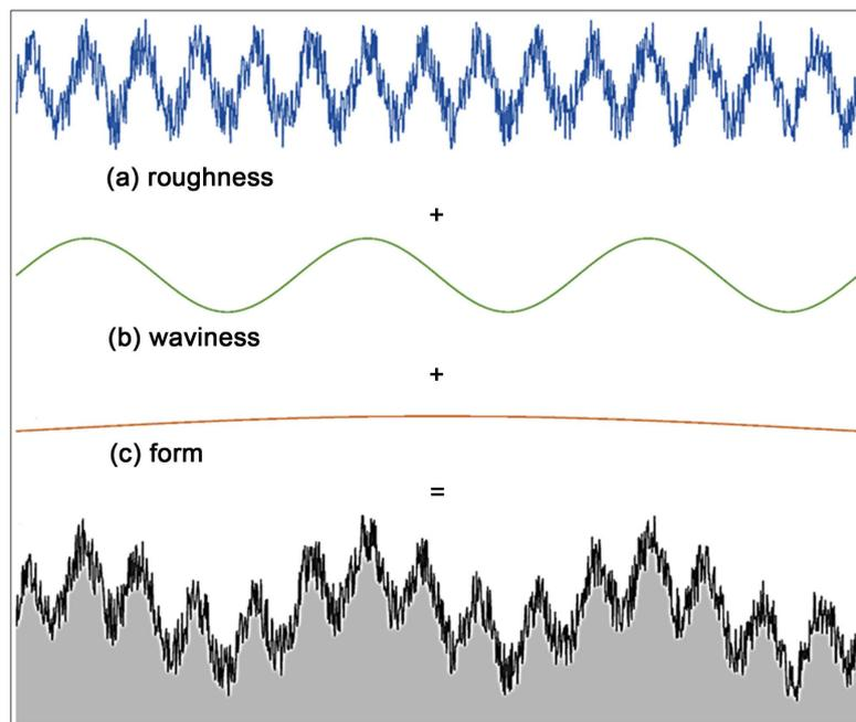
**Figure 1.** Geometric components of a surface profile: (a) roughness; (b) waviness and (c) form.
