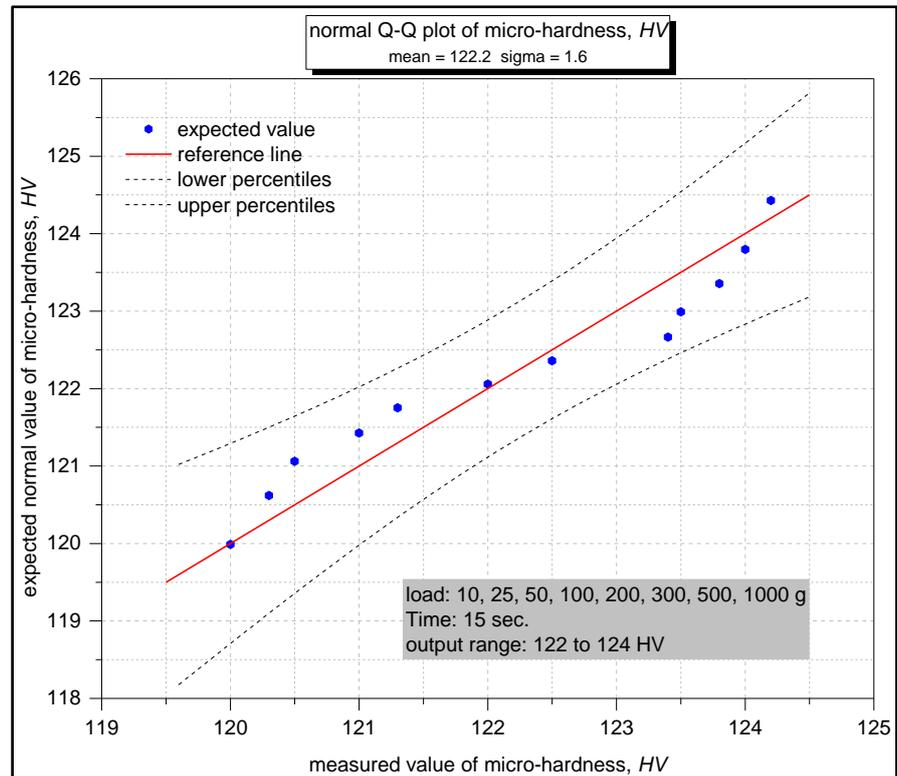
**Figure 8.** Normal Q-Q plot for micro-hardness values of Carrara marble.
