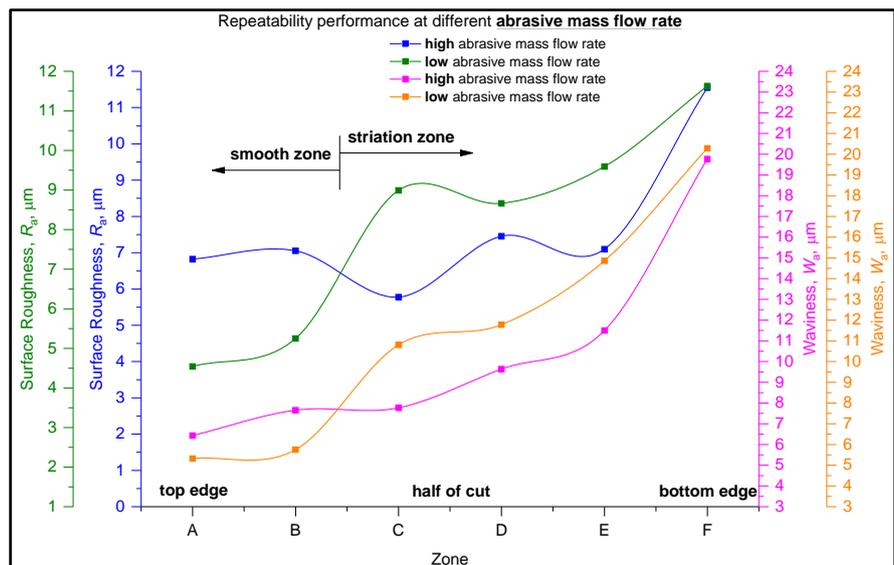
Figure 6. Effect of different abrasive mass flow rate on the surface roughness and waviness of Carrara marble.
