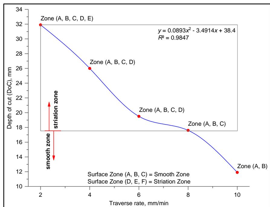
**Figure 7.** Depth of cut vs. traverse rate.
