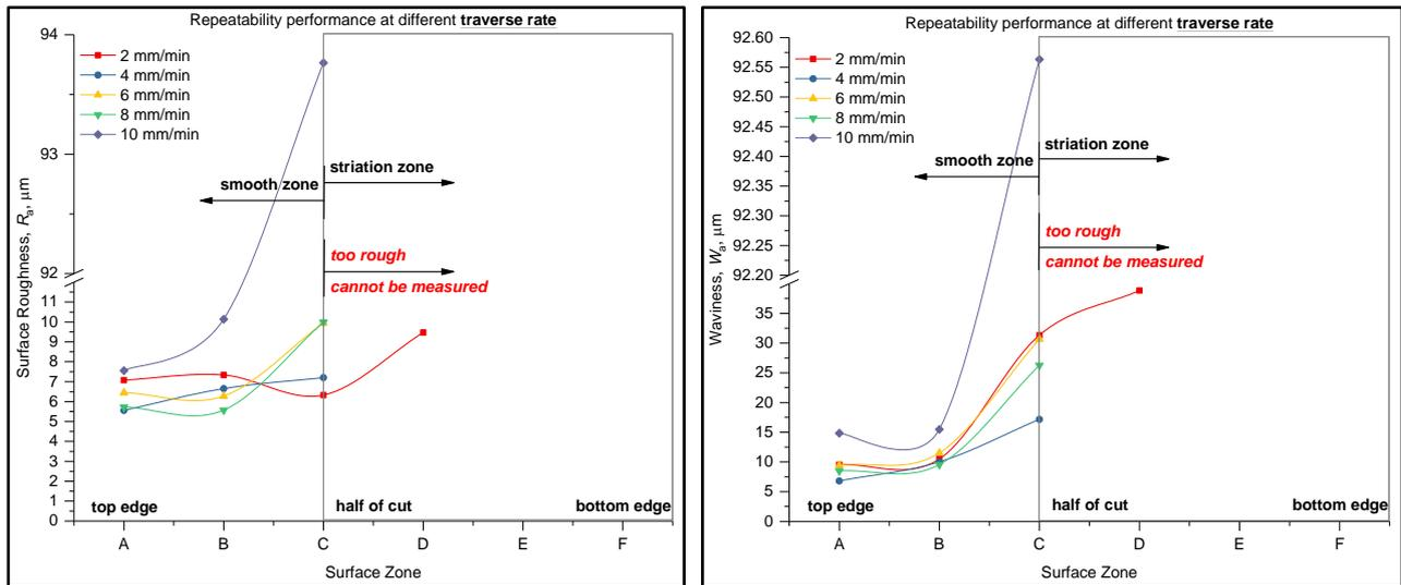
Figure 5. Effect of different traverse rate on the surface roughness and waviness of Carrara marble.
