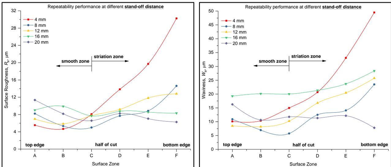
Figure 4. Effect of different stand-off distance on the surface roughness and waviness of Carrara marble.
