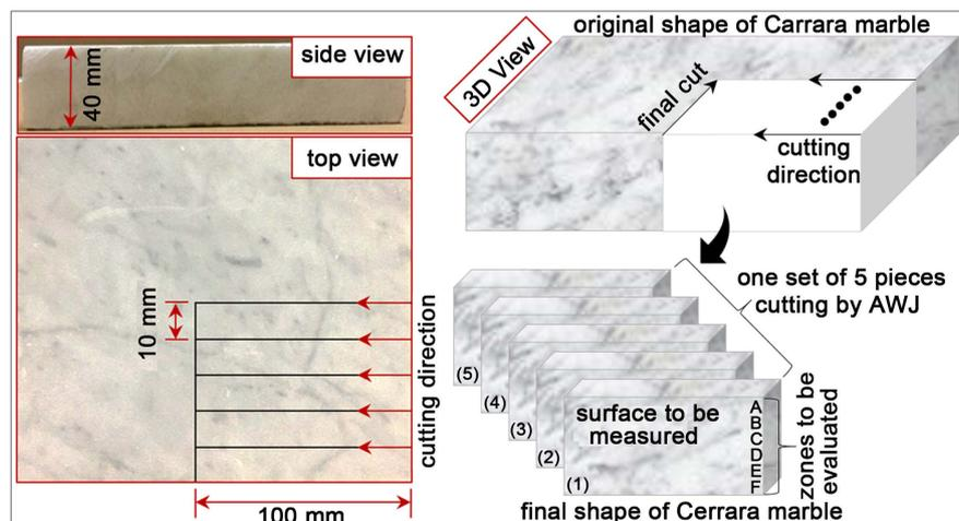
**Figure 2.** Illustration of AWJ cutting on Carrara marble.
