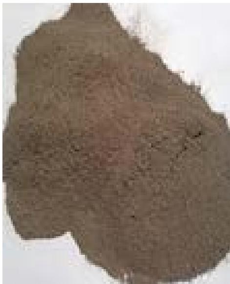
**Figure 1.** Fully-crushed oil shale.
