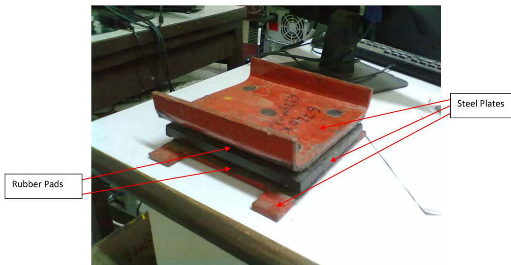
Figure 1. The three-dimensional diagram of an elastomeric pad.
