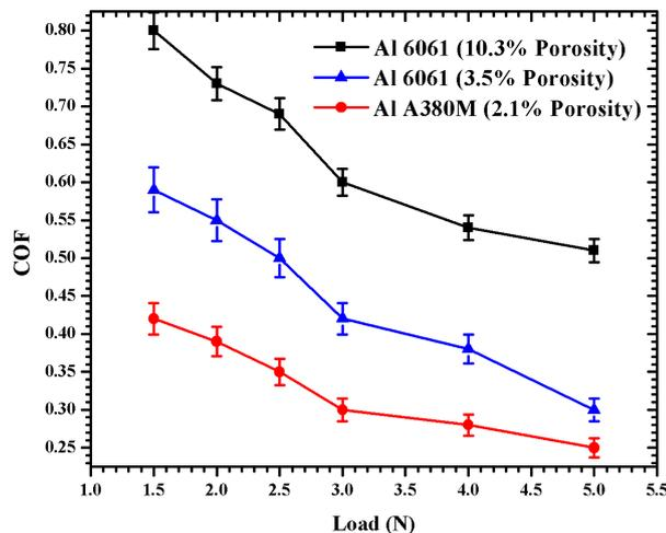
**Figure 8.** Coefficient of friction vs load as a function of porosity at 10 Hz frequency.
