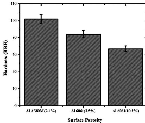
**Figure 3.** Variation in hardness with surface porosity for A380M Al and 6061Al.
