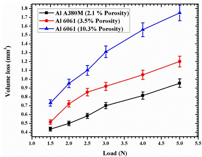
**Figure 10.** Variation in volume loss as a function of applied load for Al 6061 and A380M alloy at 10 Hz frequency.
