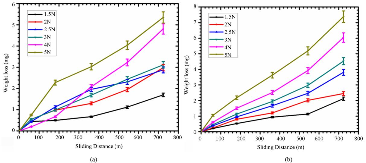
Figure 5. Weight loss versus sliding distance curve for (a) Al A380M and (b) Al 6061 (3.5% porosity).
