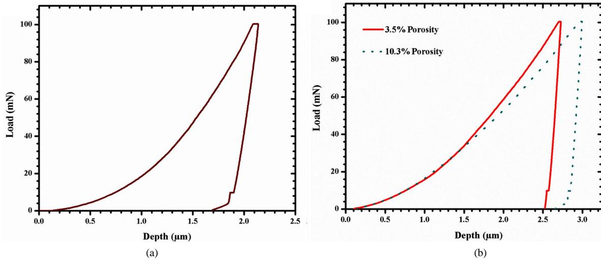
Figure 4. Load vs depth profile for (a) A380M Al and (b) 6061 Al using a max load of 100 mN.
