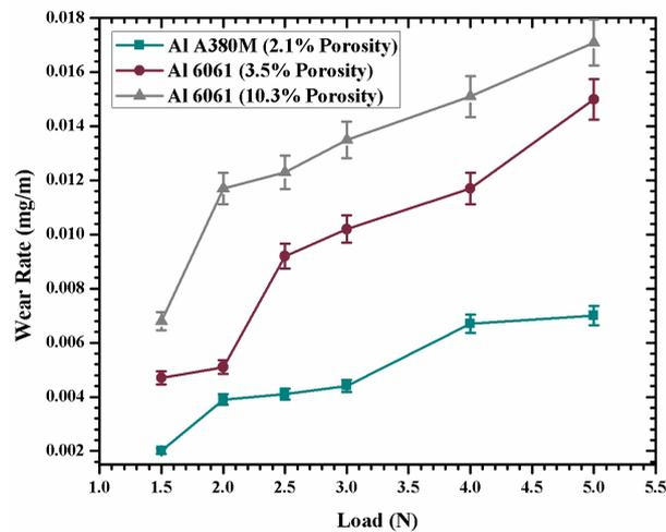
**Figure 6.** Wear rate versus normal load as a function of porosity at 10 Hz frequency.
