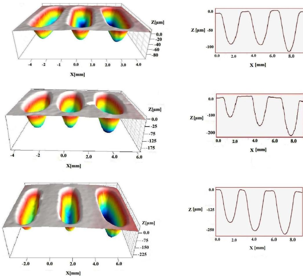
**Figure 9.** Optical profilometry scans of wear tracks. (a) (b) Al A380M; (c) (d) Al 6061 (3.5% porosity) and (e) (f) Al 6061 (10.3% porosity) at 3, 4 and 5 N load and 10 Hz frequency.
