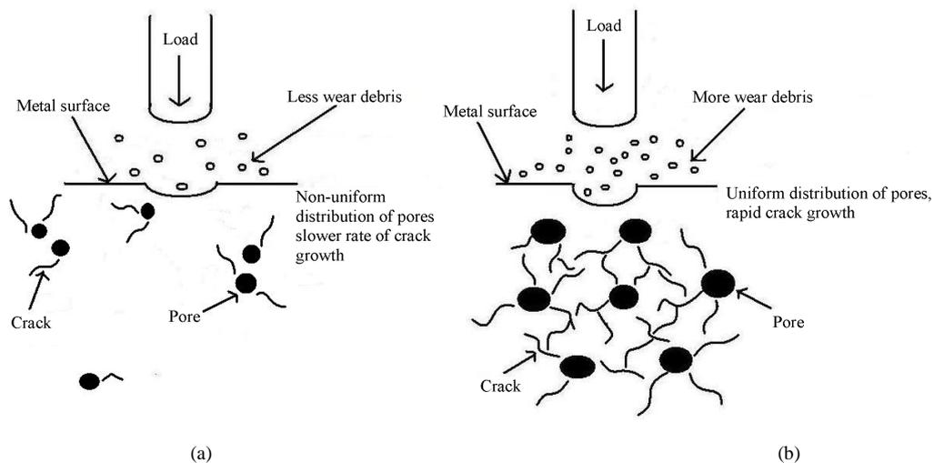
**Figure 7.** Schematic diagram depicting the effect of (a) non-uniform and (b) uniform pore distribution on wear rate.
