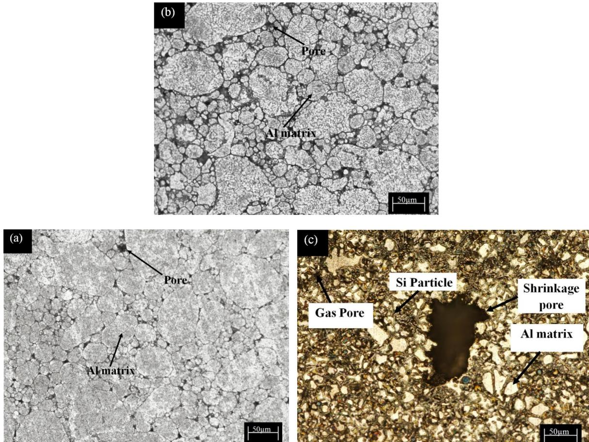
**Figure 2.** Optical micrographs of (a) sintered 6061 Al without wax (b) sintered 6061 Al prepared using 1.5% wax (c) HPDC A380M Al.
