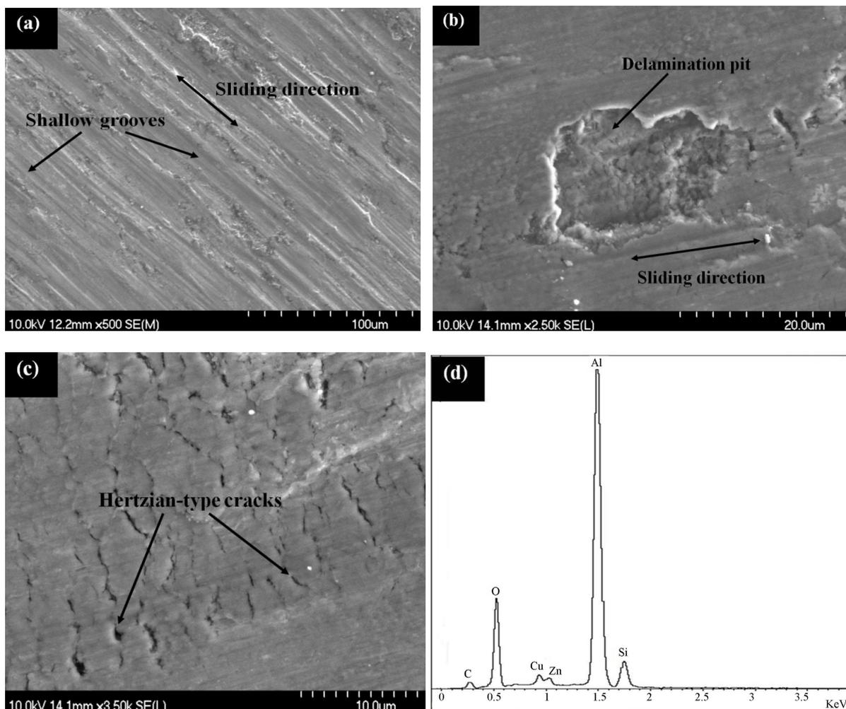
**Figure 11.** SEM micrographs of Al A380M wear track at 2.5 N load and 10 Hz. (a) Shallow grooves on the wear track; (b) Delamination pit; (c) Hertzian type cracks on the worn surface; (d) EDS analysis of the worn surface.
