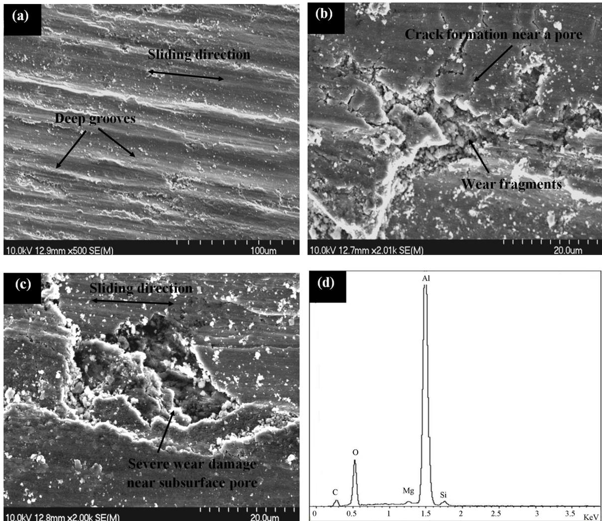
**Figure 12.** SEM micrographs of Al 6061 (10.3% porosity) wear track at 2.5 N load and 10 Hz. (a) Deep grooves on the wear track; (b) Crack initiation near a pore; (c) Wear damage near a subsurface pore; (d) EDS analysis of the worn surface.
