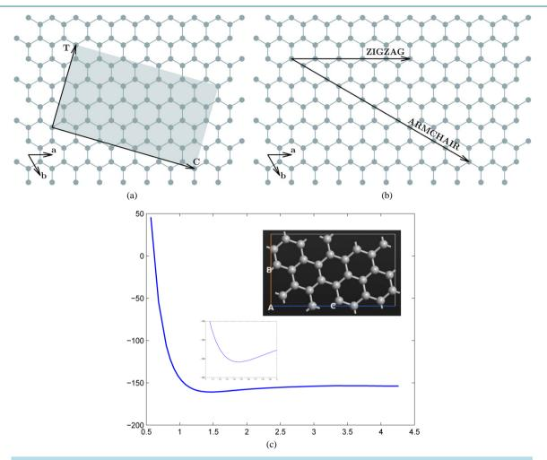
Figure 1. (a) Nanosheet: chiral vector C and translational vector T; (b) Armchair and Zigzag graphene; (c) Ground state energy for graphenes. Confining and enlarging the volume of the graphenes.
