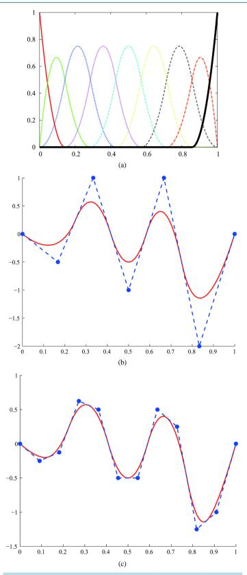
**Figure 3.** (a) B-spline bases; (b) Original B-spline; (c) a finer B-spline which has the same parametrization as the original B-spline.
