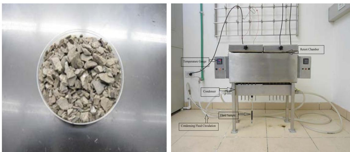
**Figure 4.** Crushed sample for oil shale and put in the retort at different temperatures.
