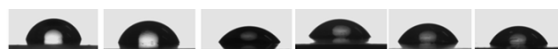
S4. The change of the contact angle of grafted PMMA surfaces [reaction time: 2, 4, 6, 8, 12, 24hours from the left].
