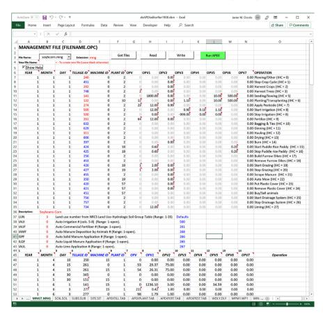
**Figure 9.** Management file worksheet depicting the help feature enabled. The "Show Help" feature allows users to view the different field operations that APEX is able to simulate and copy these to their management operations schedule.
