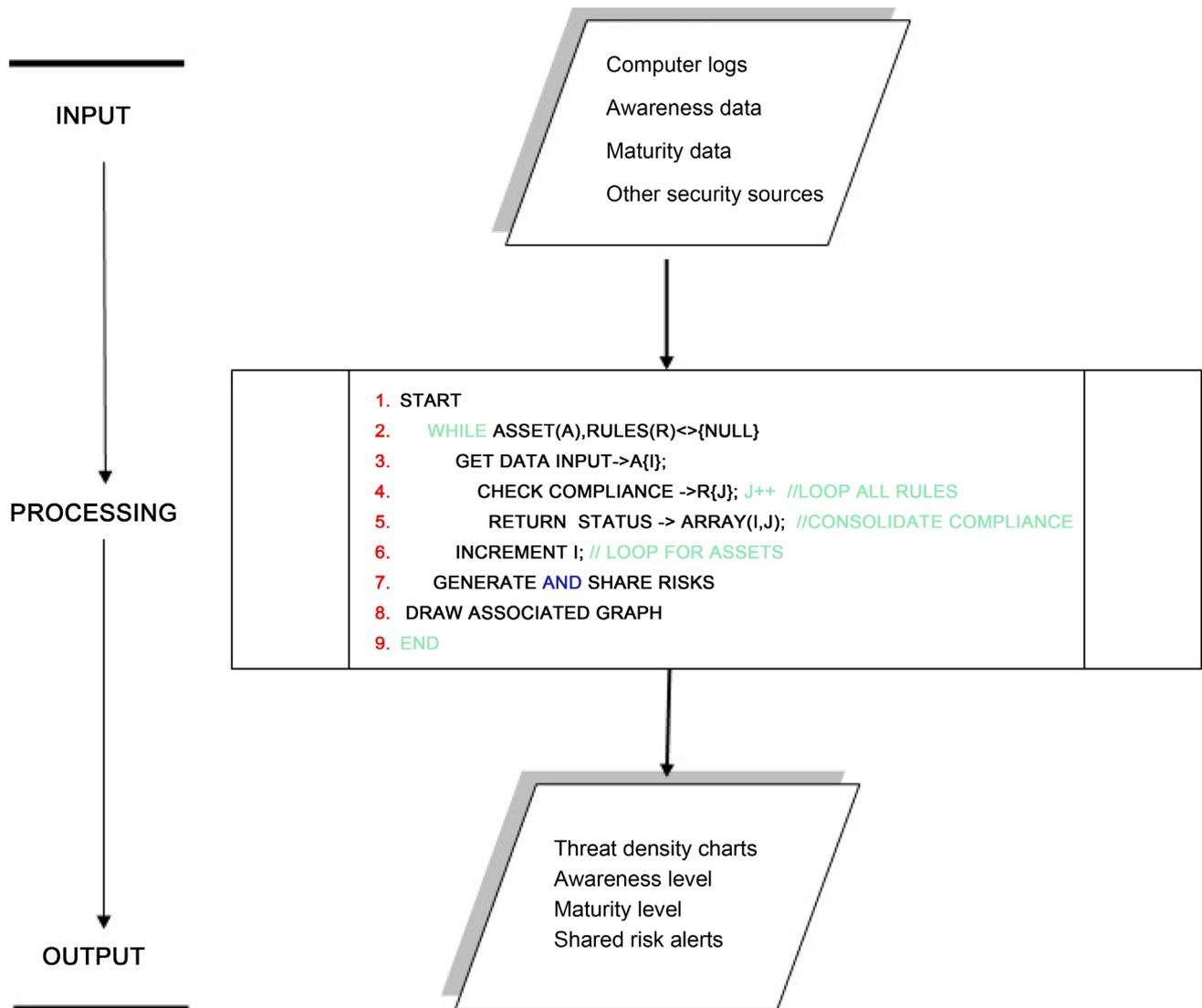
Figure 8. The analytic processing block-diagram.
