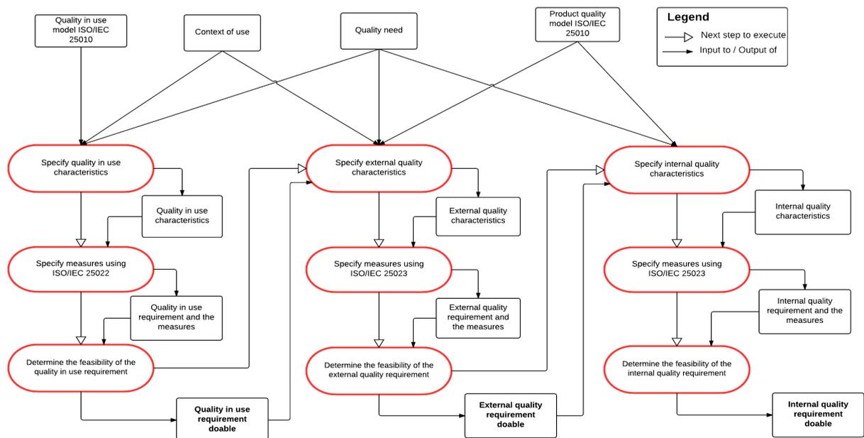
Figure 4. Process to specify and decompose software quality requirements.
