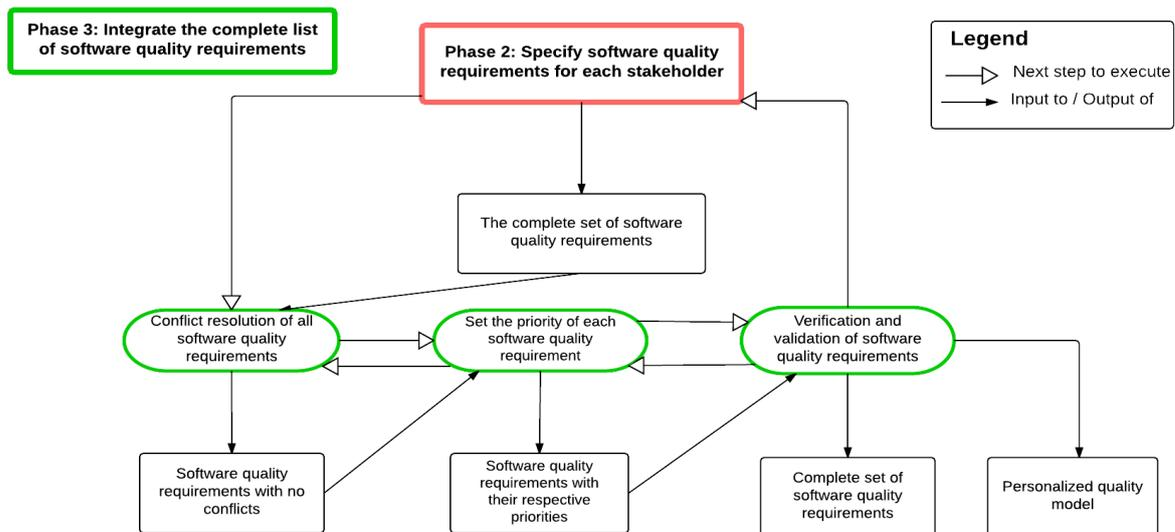
Figure 5. Process to integrate the complete list of software quality requirements.
