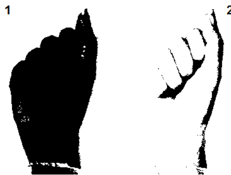
Figure 9. Difference between binary image with (1) Graythresh level ( \sim 0.7 ) and (2) Level = 0.3.
