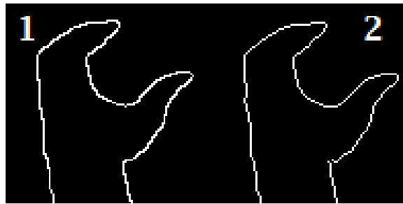
Figure 14. Edge difference between Canny (1) and Sobel (2) in a binary image.
