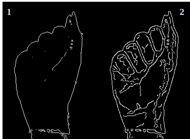
Figure 12. Edge difference between Sobel method (1) and canny method (2).
