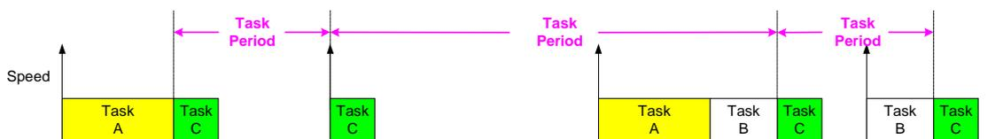
Figure 3. Release jitter caused by task placement in TTC schedulers.
