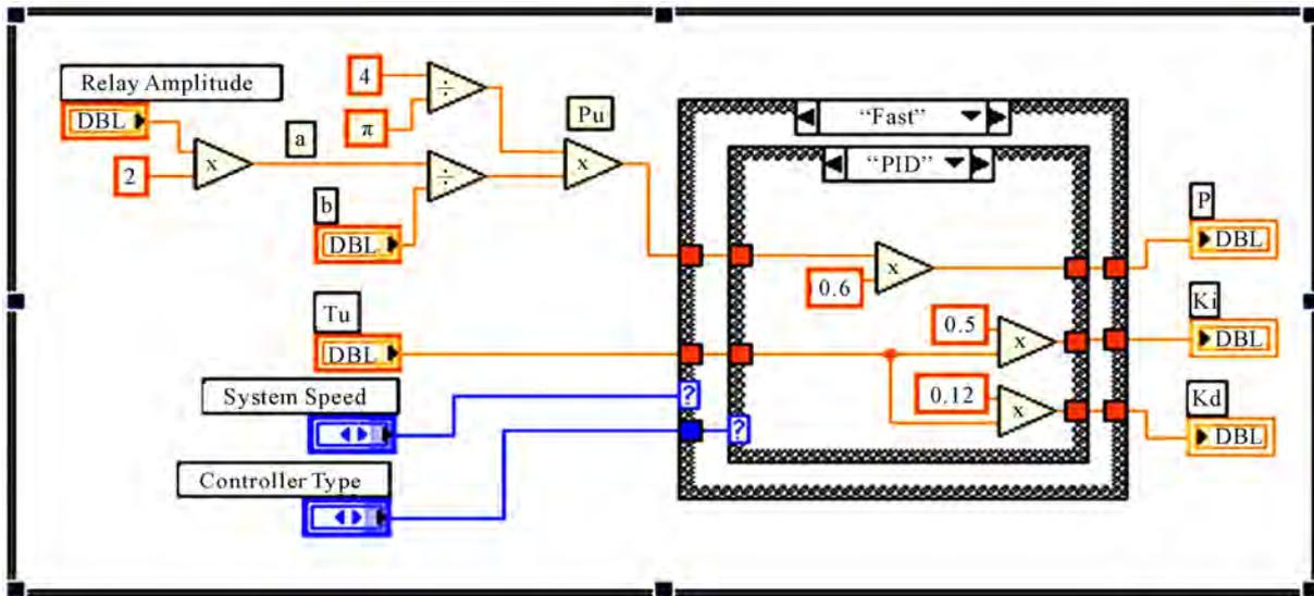
Figure 9. Calculate best PID parameters block diagram.
