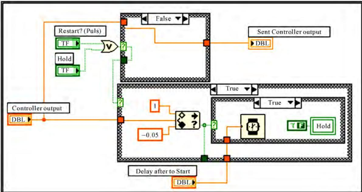
Figure 7. Restart response block diagram.
