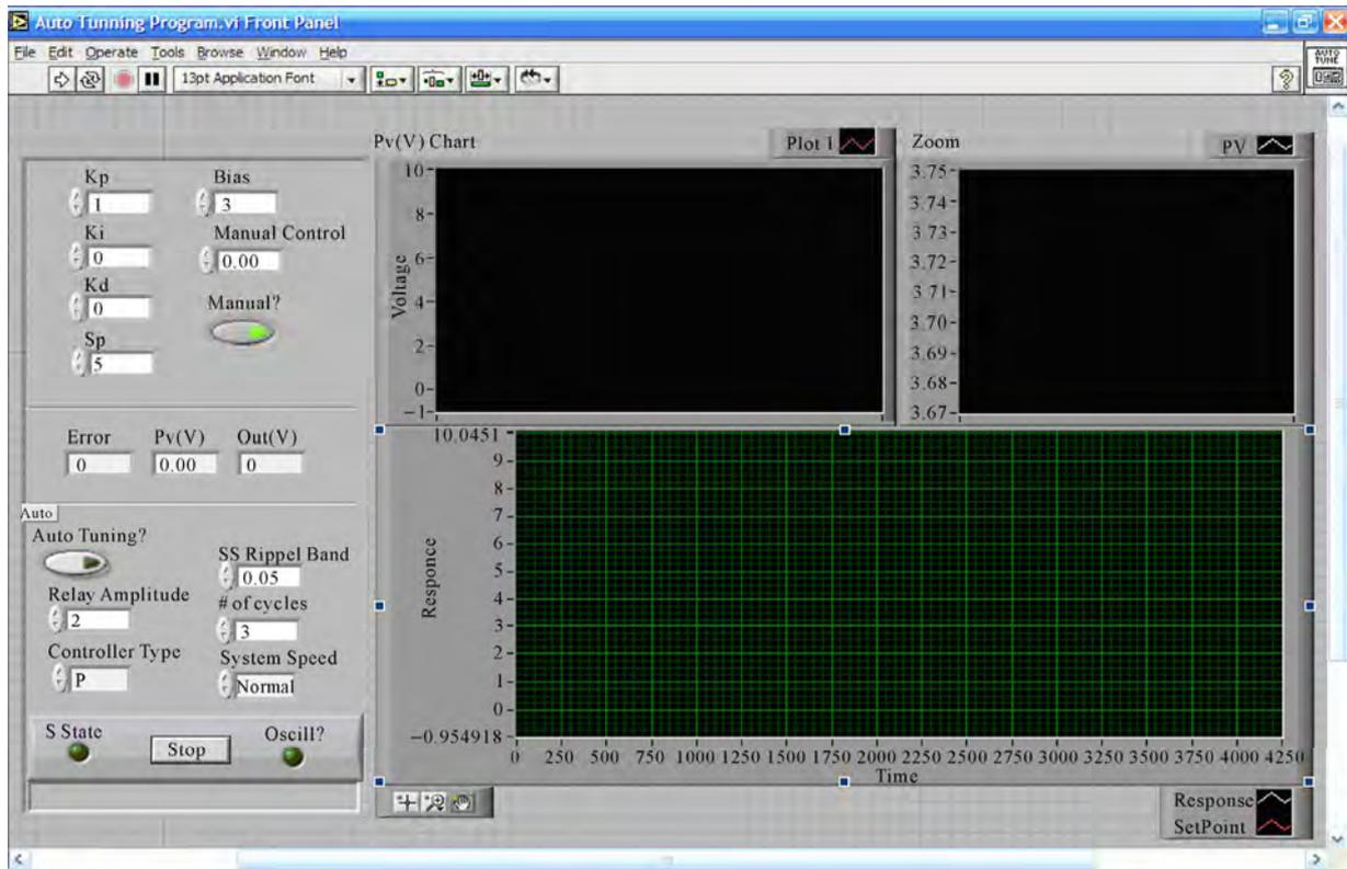
Figure 3. The front panel of PID auto-tuning VI.
