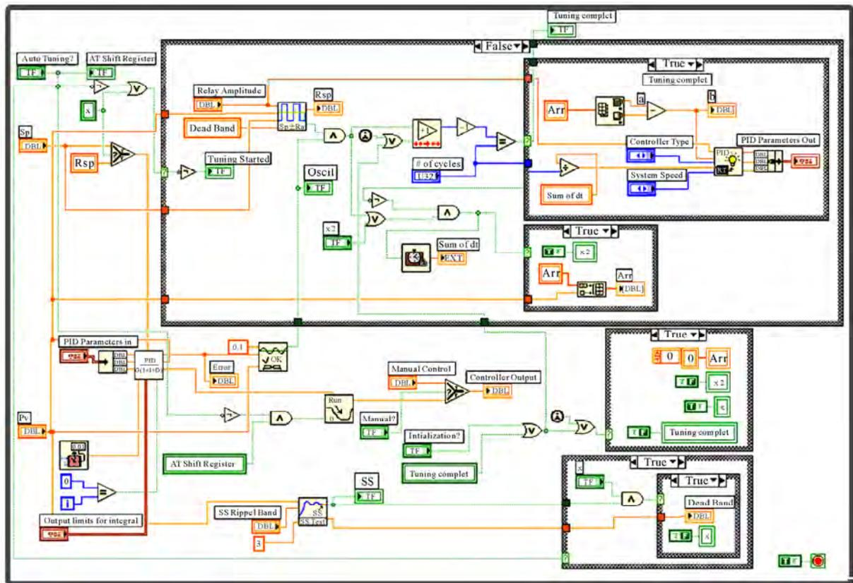
Figure 6. PID auto-tuning (all features) block diagram.
