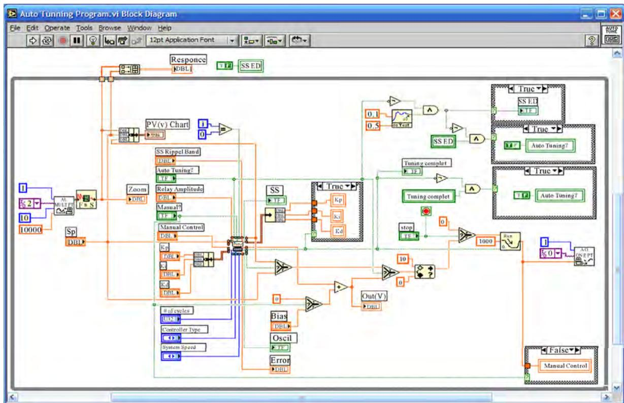
Figure 4. PID auto-tuning VI block diagram.
