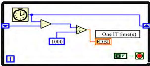
Figure 11. Find iteration time (dt) block diagram.
