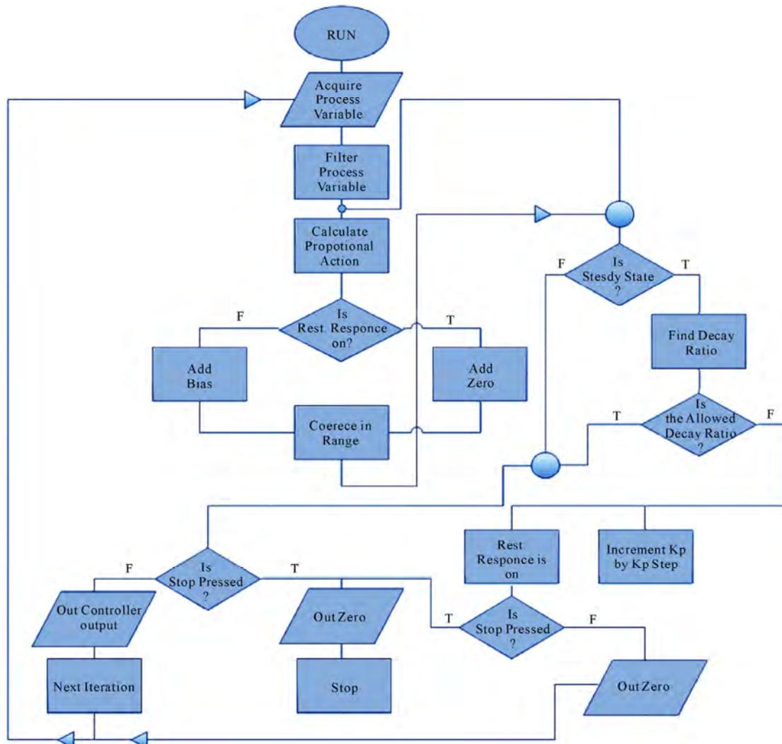
Figure 2. PID auto-tuning VI flow chart.
