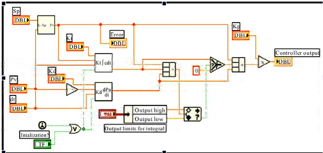
Figure 13. PID controller block diagram.
