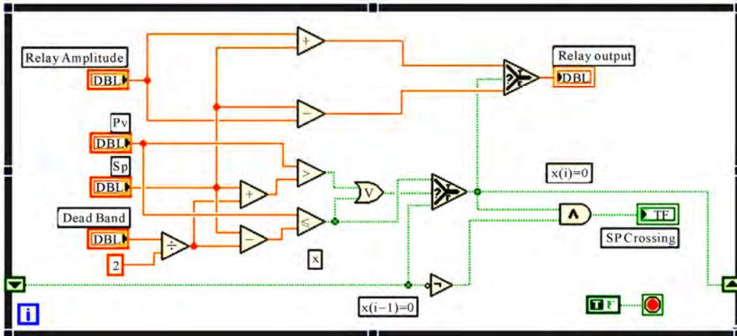
Figure 12. SP relay block diagram.
