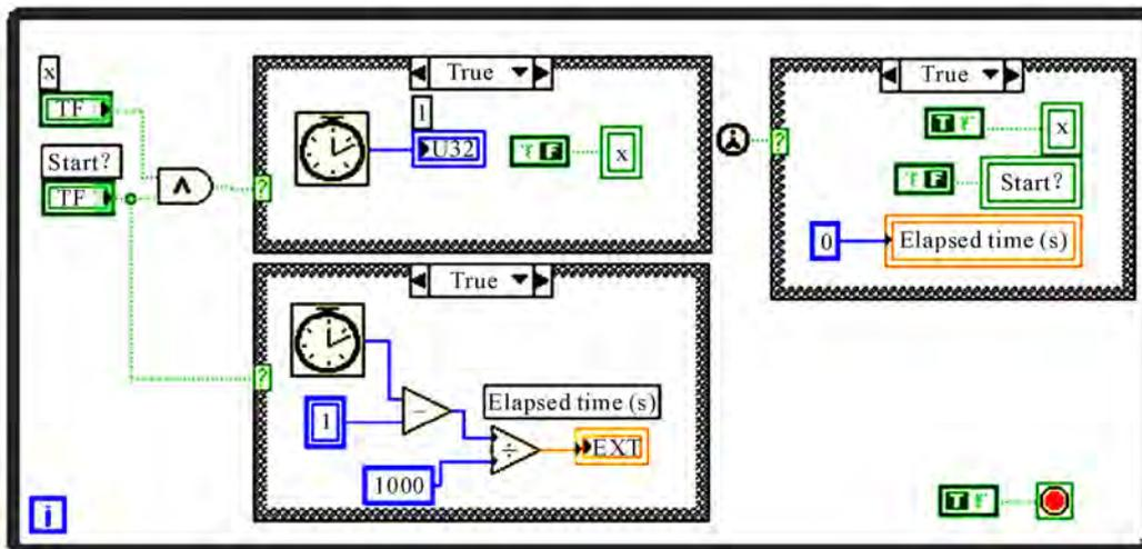
Figure 14. Stop watch block diagram.
