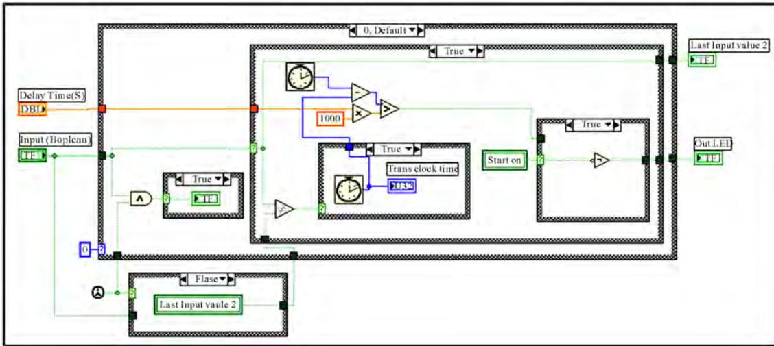
Figure 1. On-delay timer block diagram.
