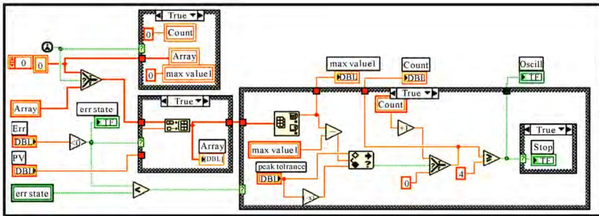
Figure 10. Check oscillation block diagram.
