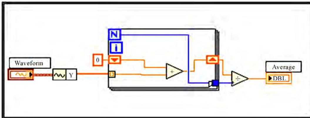
Figure 16. Waveform values average block diagram.
