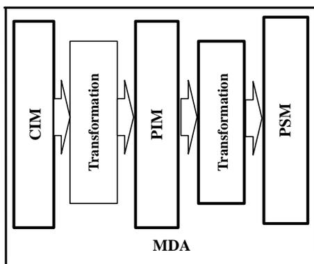
**Figure 1. Model Driven Architecture.**
