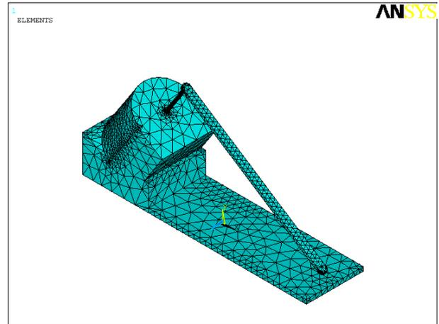
**Figure 8. FE model of the motor assembly.**
