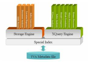
Figure 5. The architecture of TV-anytime metadata management system
