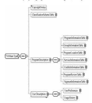
Figure 1. The structure of TV-Anytime Metadata
