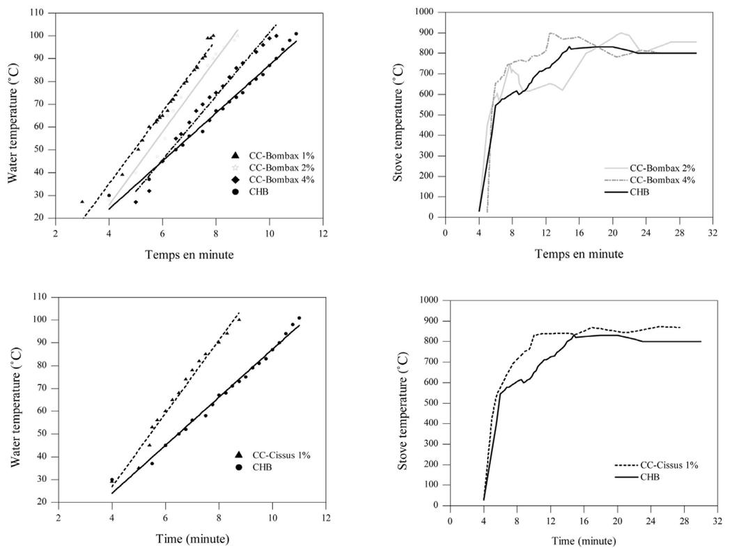
**Figure 4.** Temperatures profiles for water and in the stove for Corn Cobs briquettes.
