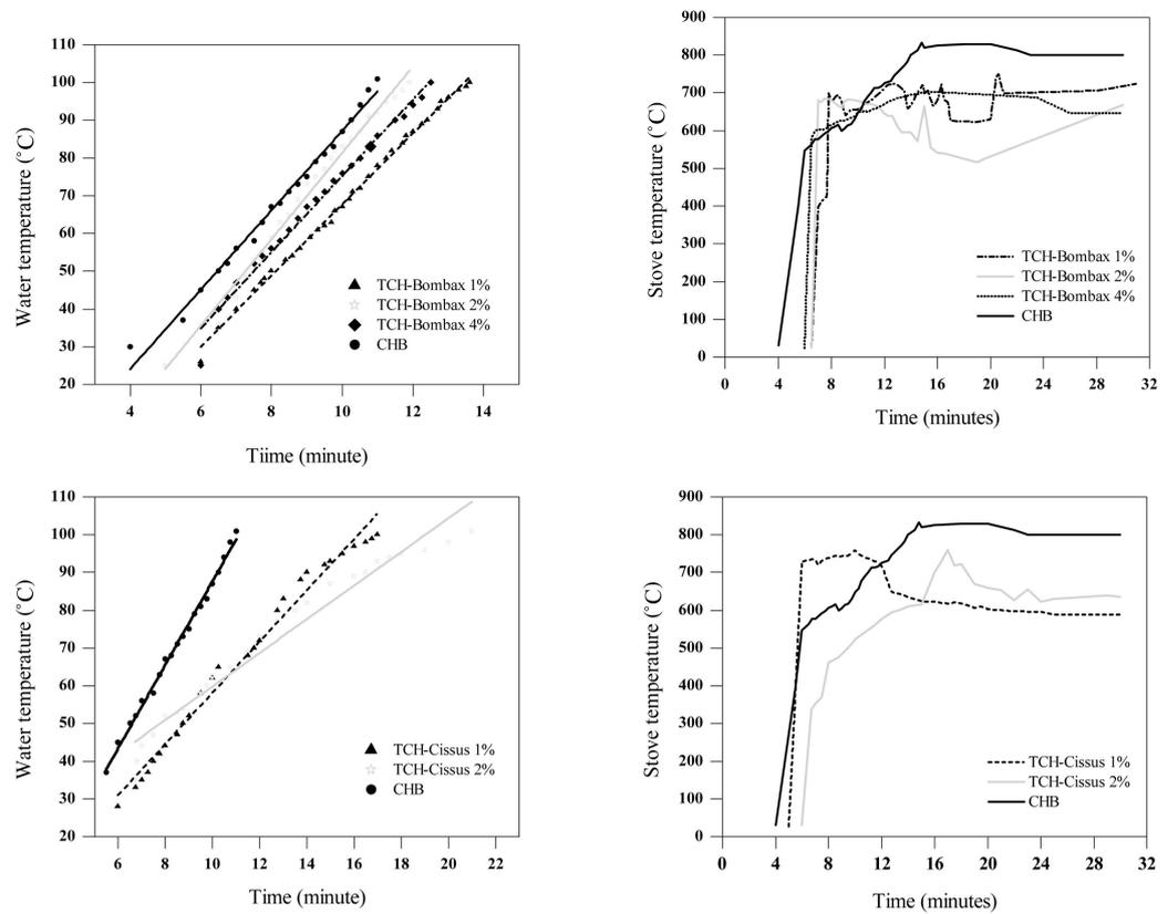
**Figure 3.** Temperatures profiles for water and in the stove for Coconut chars briquettes.
