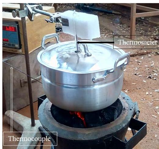
**Figure 2.** Experimental apparatus for energy efficiency tests.
