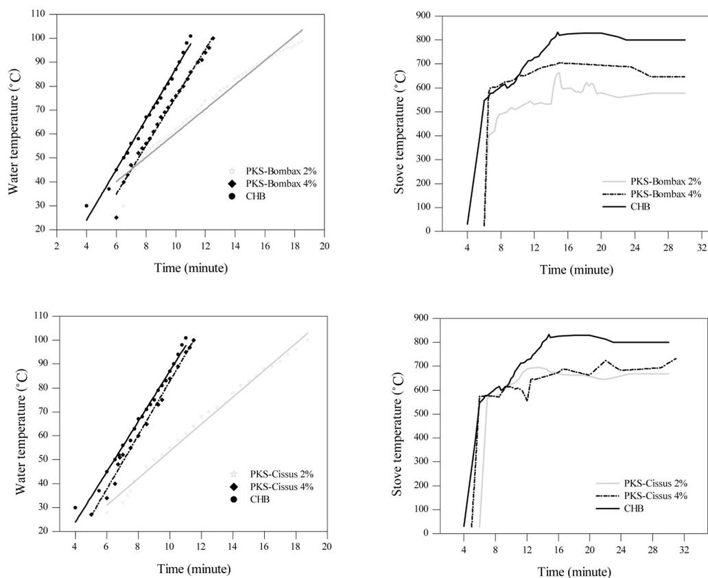
**Figure 5.** Profiles of temperatures of water and in the stove for Palm Kernel Shell briquettes.
