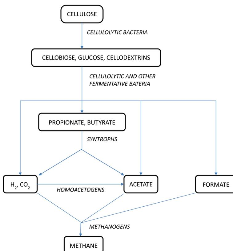
**Figure 3.** Diagrammatic representation of anaerobic cellulose degradation by microbial communities. Formate, volatile fatty acids (acetate, propionate, butyrate), CO<sub>2</sub>, methane are major fermentation products. Lactate, succinate, and ethanol are also produced by fermentative microorganisms but usually do not accumulate [28].
