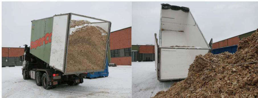
Figure 5. The composite container before unloading on the left and after on the right.
