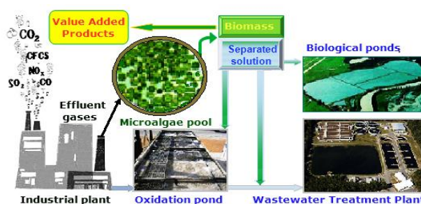
Figure 1. Vision on application of microalgae for purification of industrial wastewater and gas effluent as well as improvement municipal wastewater treatment in wastewater treatment plant.
