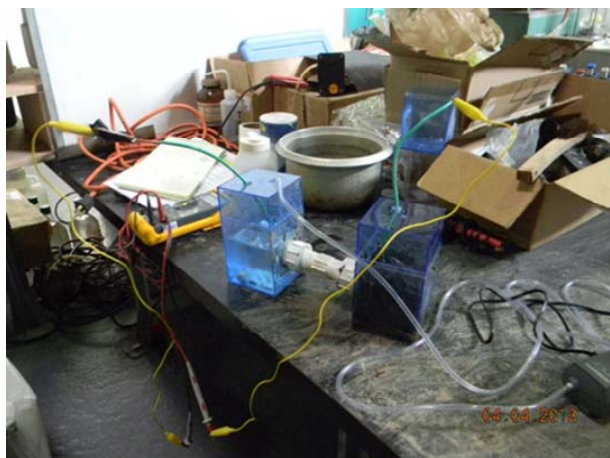
Figure 2. Picture of MFC system setup.
