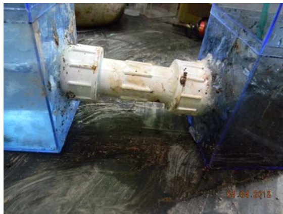
Figure 5. Picture of anode, cathode chambers and salt bridge.
