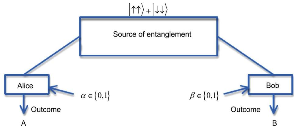
**Figure 2.** The operation principle of the proposed QKD protocol. An entanglement source produces a pair of entangled signals, which are randomly measured in certain bases chosen by Alice and Bob separately. Alice and Bob generate outcomes  $A$  and  $B$  respectively.
