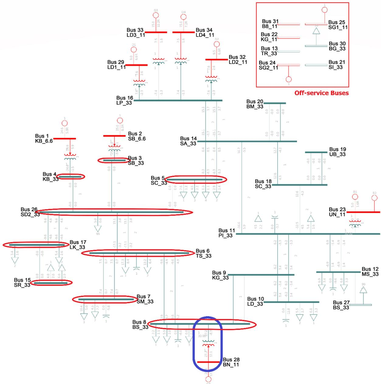
**Figure 3.** N-1 case with affected buses when outage of transformer branch from bus 8 to bus 28.
