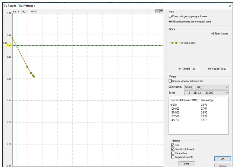
**Figure 5.** Maximum additional power transfer at 0.9 pu in PV curve.
