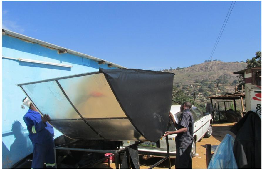
**Figure 11.** Side walls of the four wing CPC collectors wrapped with polyethylene sheets to preserve heat.
