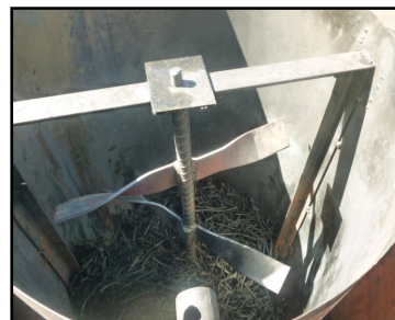
Figure 7. Inside of the reactor with produced biochar.
