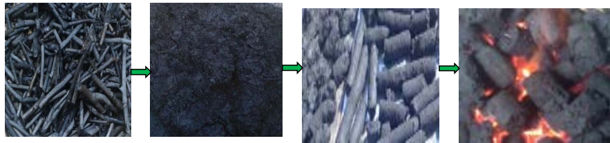
Figure 9. Produced biochar before compaction, mixing, briquette and combustion of biochar [21].
