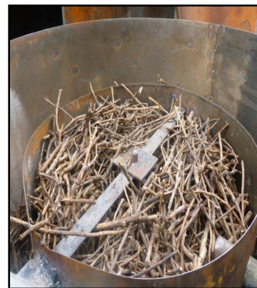
Figure 6. Inside of the reactor before covering.
