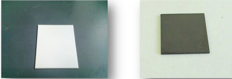
**Figure 1.** (a) Alumina tile; (b) Ni/YSZ coated sample.
