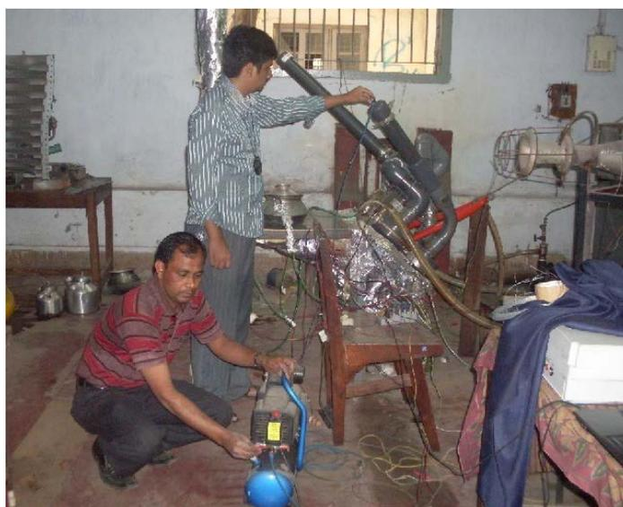
**Figure 3.** Pressurizing the system with compressed air.
