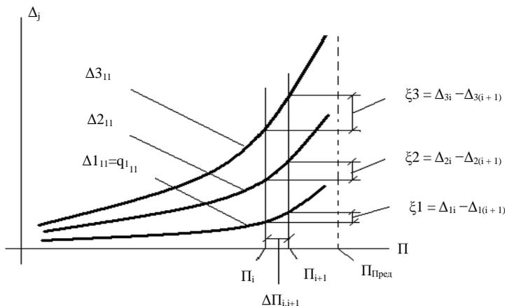
**Figure 3.** Definition of the steady-state stability simplified criterion for the complex EPS ( $\Pi$  is the operating condition parameter of EPS).
