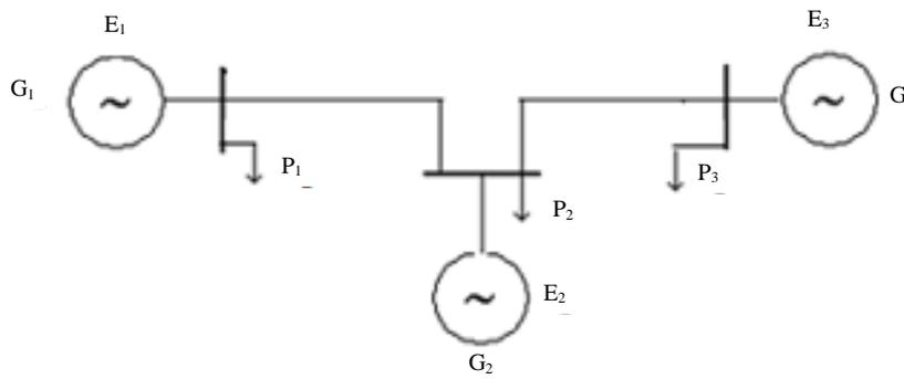
**Figure 2.** The circuit design of three-generator electrical power system.
