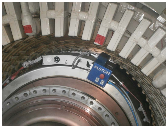
Figure 3 DIRIS Small air gap robot deployed on a 175 MW generator of North American manufacturing origin.
