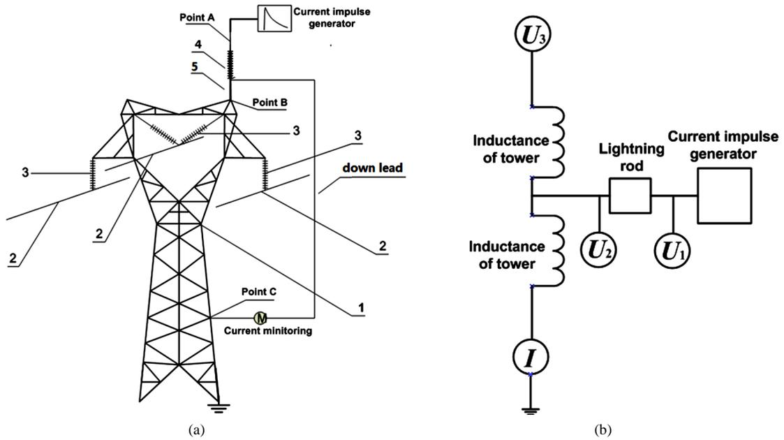
**Figure 4.** The test circuit (1—the tower; 2—transmission lines; 3—the insulators; 4—the lightning rod; 5—the insulated support). (a) the 500 kV tower; (b) the equivalent circuit.
