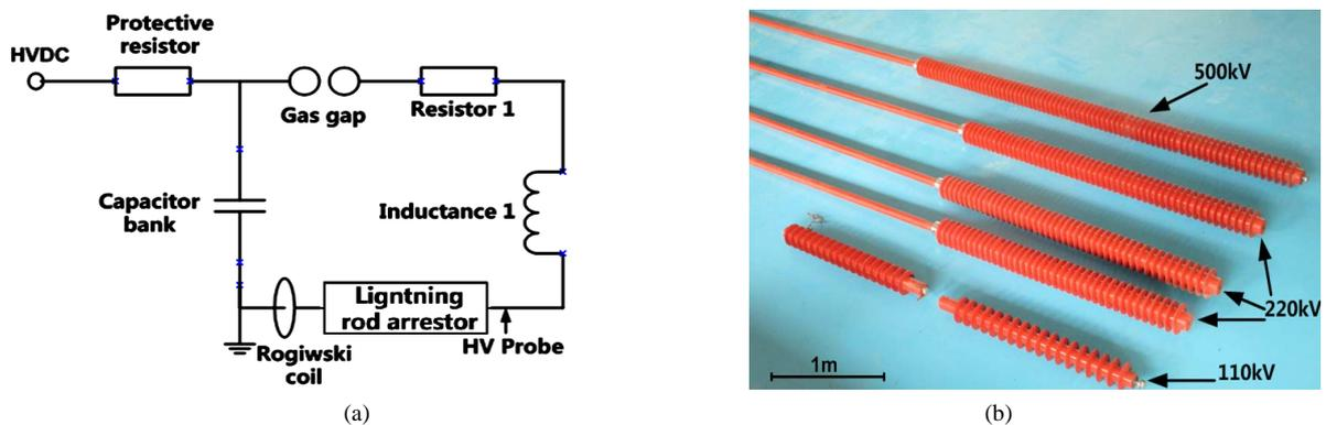
**Figure 1.** The schematic of the test circuit and the picture of lightning rod arresters. (a) test circuit; (b) lightning rod arresters.
