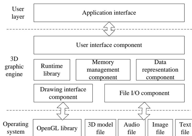
**Figure 2.** Structure of the 3D graphic engine.
