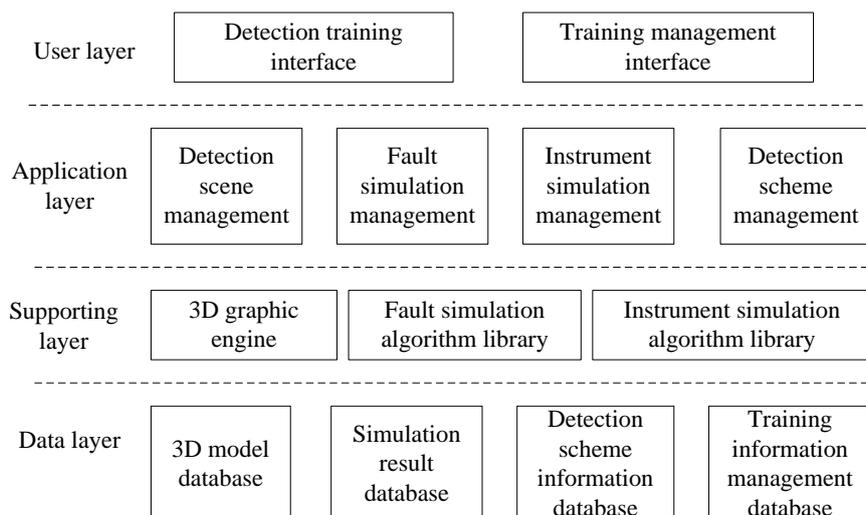
**Figure 1.** Architecture of the training simulation system.
